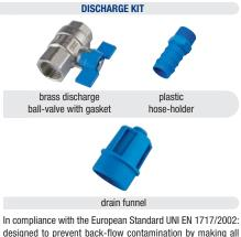
designed to prevent back-flow contamination by making all elements downstream the discharge vent to atmosphere (protection unit symbol: DC)
